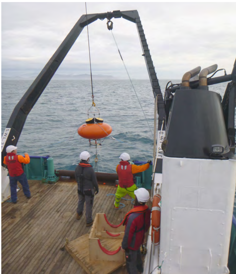
An oceanographic team aboard NIWA’s R/V Kaharoa deploying an acoustic Doppler current profiler in Cook Strait. Facing page: Te Moana-o-Raukawa to measure flow variability in the highly turbulent waters of the strait.
