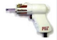
A needle free jet-injection device, likened to a Star Trek 'hydrospray', has been developed by researchers at the Auckland Bioengineering Institute (ABI) and the Massachusetts Institute of Technology (MIT) in the US.
