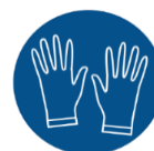
PROTECTIVE GLOVES REQUIRED
