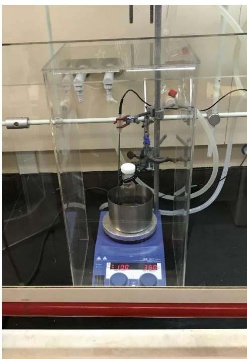
Figure 1: Ideal use and set up of a Blast Shield. Note that the combination of fully lowered fume hood sash and blast shield assist in containing any potential explosion.
