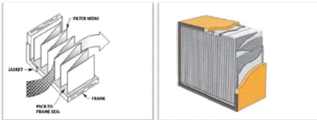
Figure 5: HEPA filter construction
